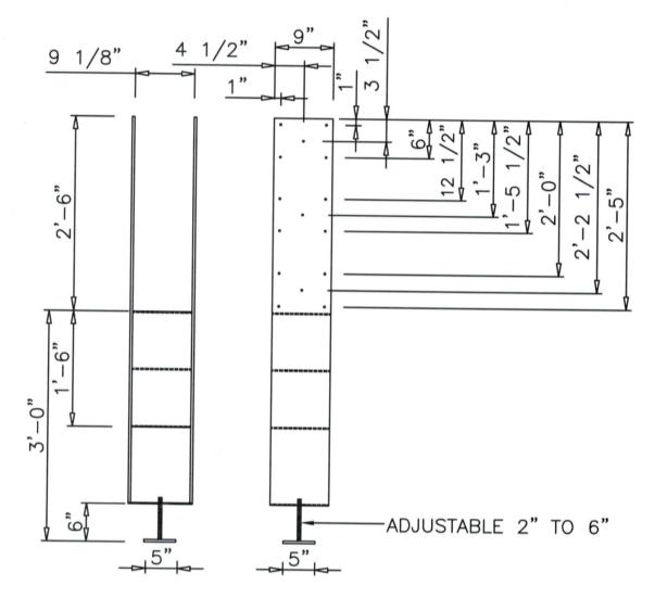
ALL HOLES 9/32" FOR SIMPSON STRONG-DRIVE SCREWS ALL PLATES 3/8" THICK, Fy = 50,000 psi STEEL PROVIDE 1" EDGE DISTANCE FOR HOLES
