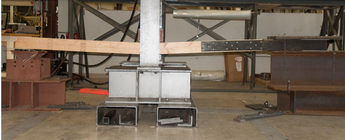
Figure A7. 2x6-4 ply shortly before failure.
