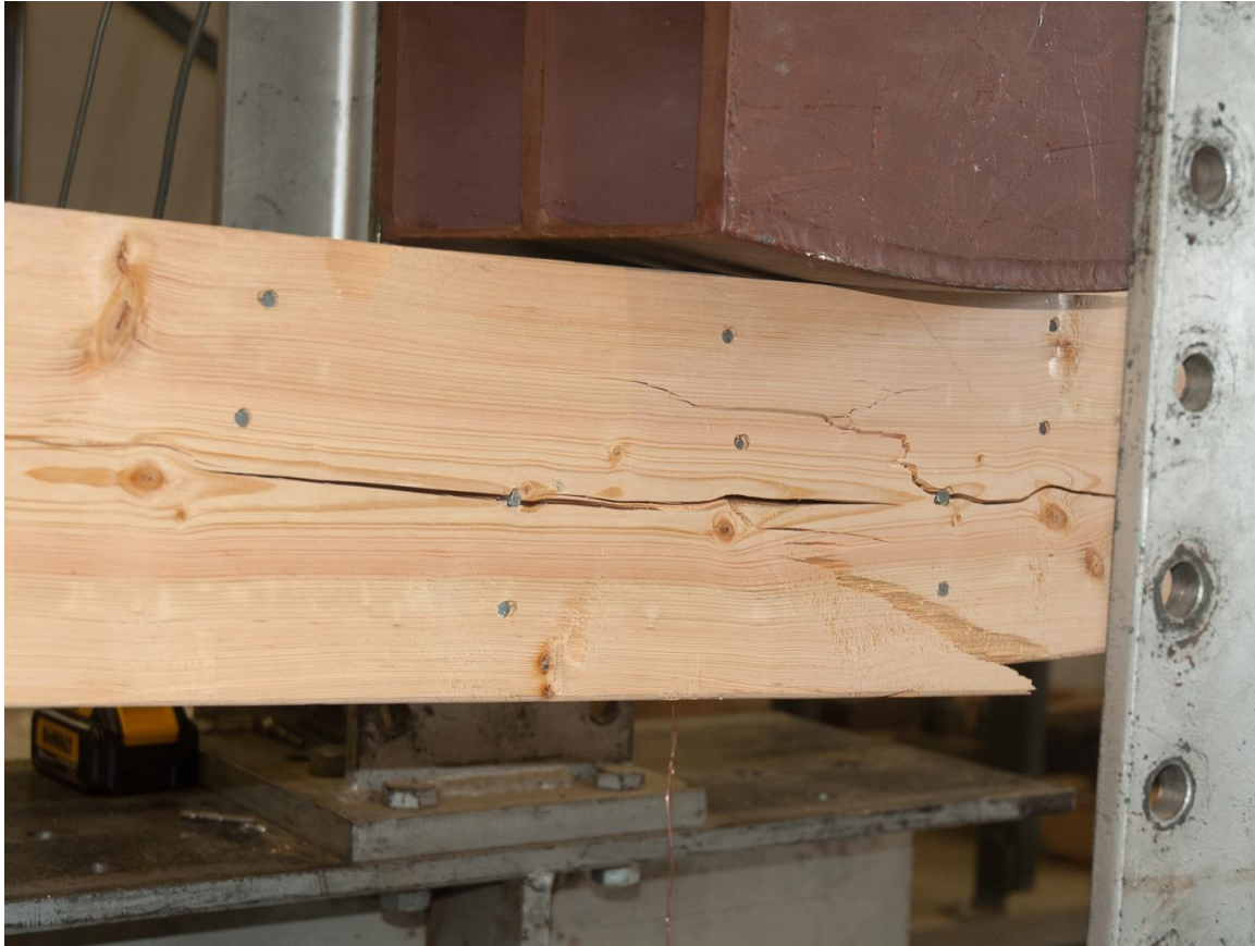
Figure A1. 2x8-4 ply bending failure initiating on tension failure.
