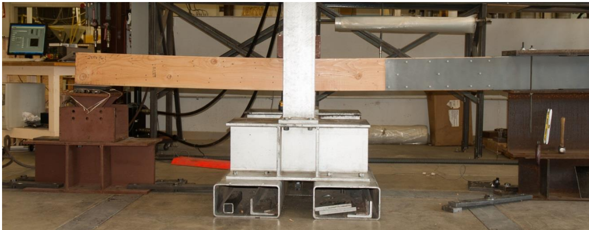
Figure A2. 2x10-3 ply shortly before failure.
