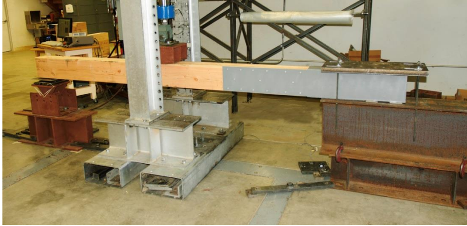
Figure 2. Typical propped cantilever test setup.
