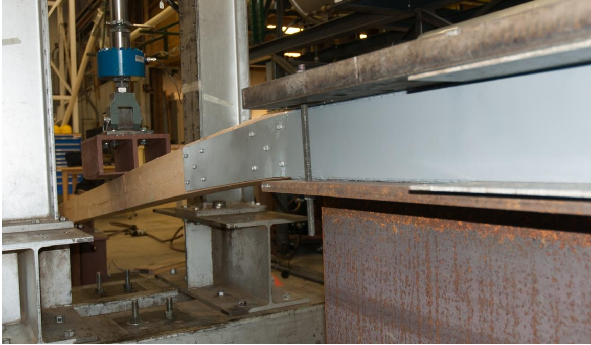
Figure A3. Cantilever after steel yielding.
