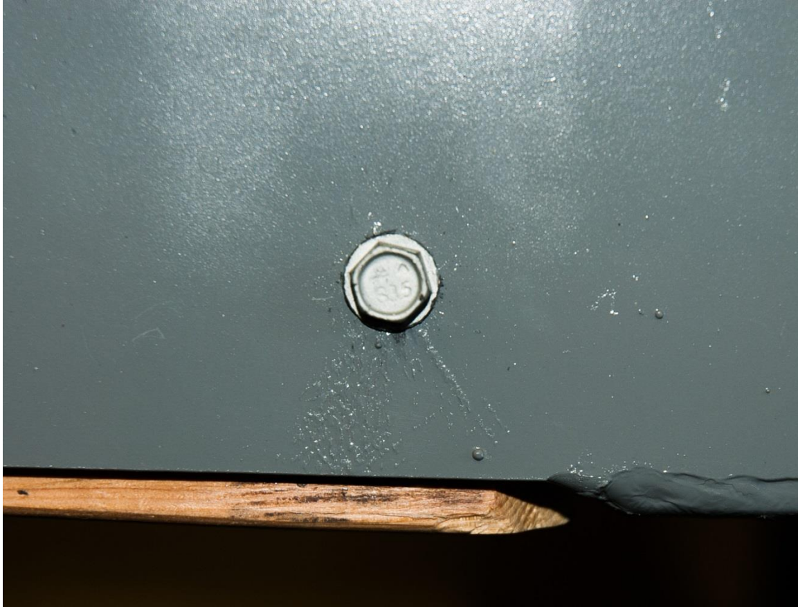
Figure A5. Yielded steel on 2x6-3 ply propped cantilever test.
