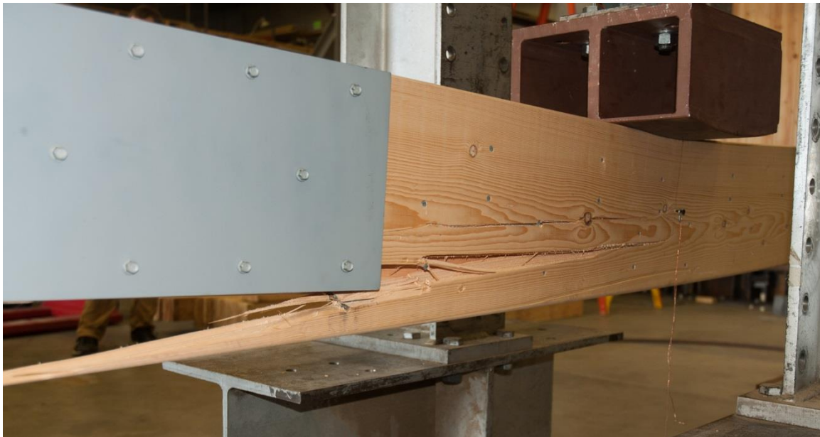
Figure A6. 2x10 3-ply splintering tension failure
